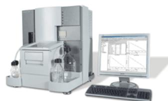
**Nanoparticle Characterization:** The [Malvern Instruments' Zetasizer ZS](#) measures particle size (0.3 nm to 10  $\mu\text{m}$ ) via Dynamic Light Scattering with backscatter optics, Zeta potential, and molecular weight (as low as 342 Dalton). Aqueous and organic solvents can be used, with samples as small as 12  $\mu\text{l}$ , and controlled temperature (0-90  $^{\circ}\text{C}$ ). **COMING SOON**
